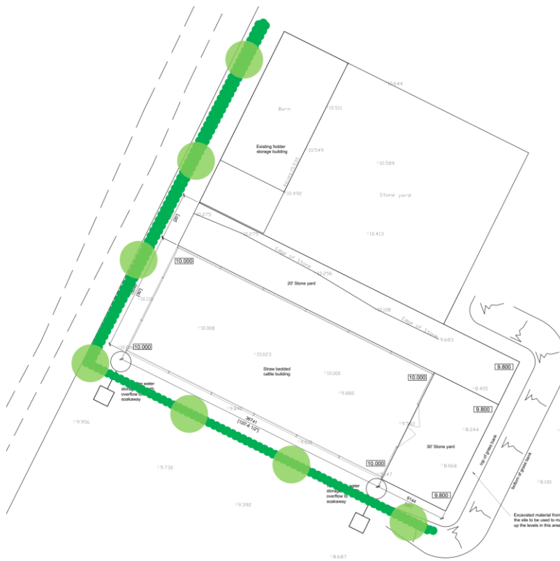
Figure 11: Visual impact mitigation required by pre-commencement condition (indicative sketch made by landscape officer).
